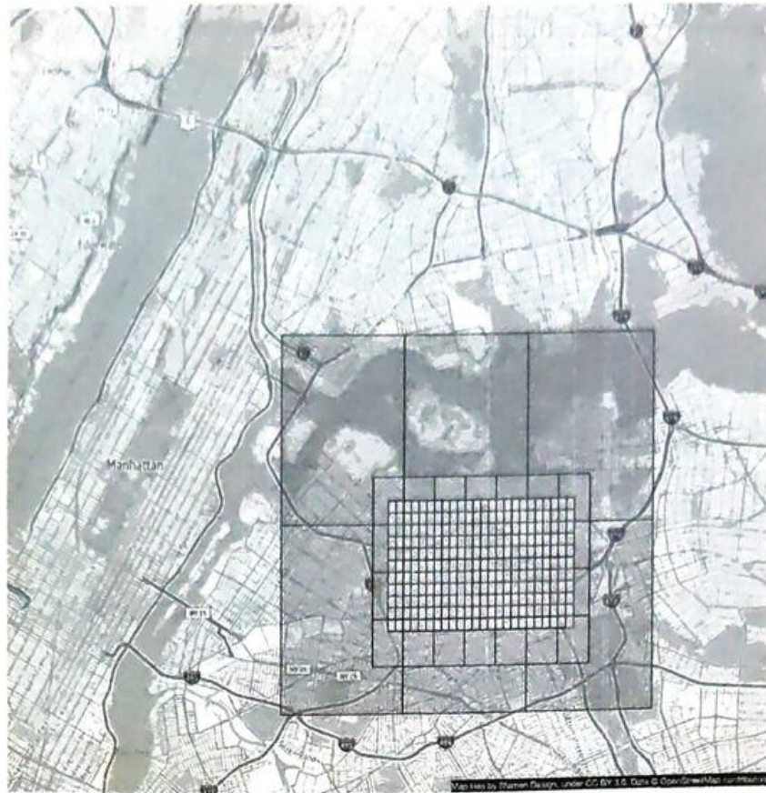
Figure 3.6: Routing tiles of varying sizes
